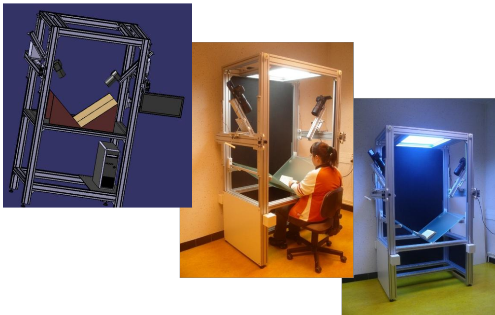
Figure 3. Self-made V-shape book scanner based on double EOS600D (18MPixel each) developed by the French partner IFMA. CAD-Model and prototype
